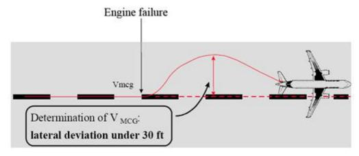
The VMCG is defined as the speed which, when one engine fails, leads to a lateral deviation of 30 ft when controlling the aircraft with aerodynamic means only.
